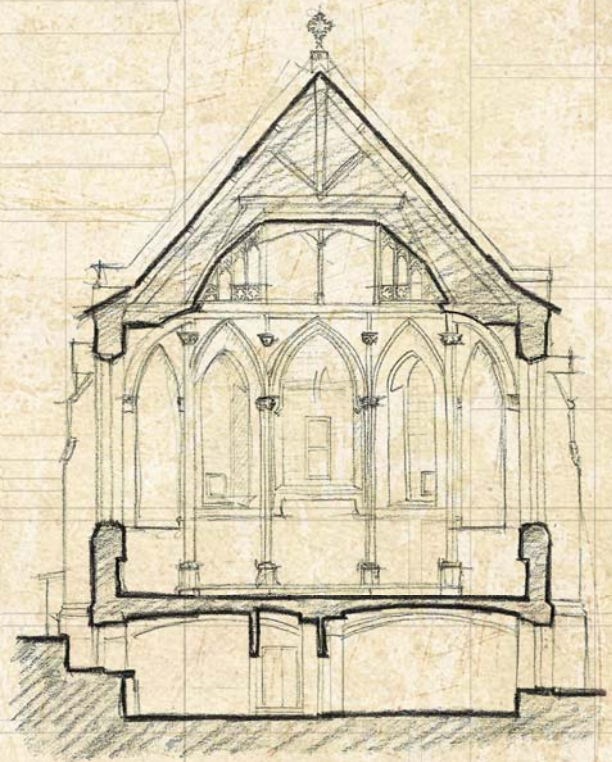
Artist's sketch of foundation reinforcement work planned for the 2019 construction season with money raised from the St Andrew's community; also repair and restoration of support structures between the ceiling and roof which would be included in a city-funded project in 2020.
